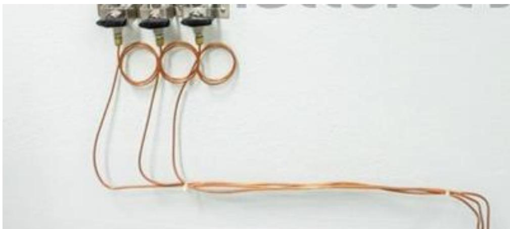
More often than not valves and fittings to the instrument may not look so neat and tidy and could be intertwined 1/8" copper tubing. Critically this may not easily identifiable if you need to isolate, leak check, or reconfigure the gases, particularly if you have restricted access around the back of the instrument. Also, any isolation valve fitted may not be secured to a fixing point or surface which on operation can lead to strain on the fittings which can result in leaks.
